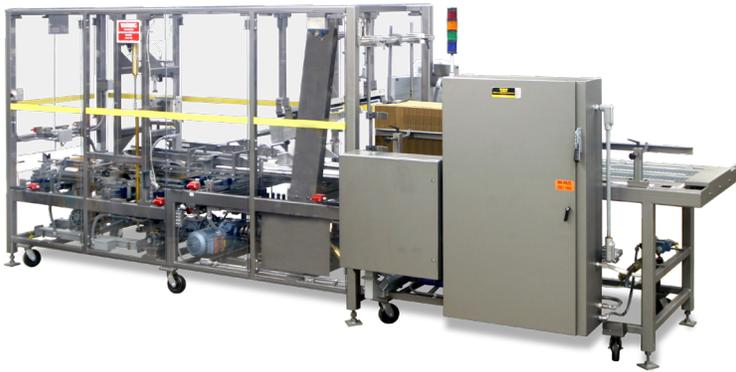
The TR-60 Fold Over Interlocking (FOIL) Tray Former produces up to 60 FOIL trays per minute for food processing, pharmaceutical, and other high-demand production lines running full- and half-sheet formats. Its mechanical pick-and-place system maintains controlled sheet handling from pickup through placement, helping keep output consistent even when material varies.
