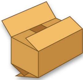
Overlap Slotted Container (OSC) In this style, the length of the box is greater than the width. The sealed overlap helps to keep the outer flaps from pulling apart. Ideal for packaging where overlap seal prevents dust ingress.
